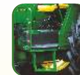
Side bar & steps with mat Climbing up and down the tractor is now easier
